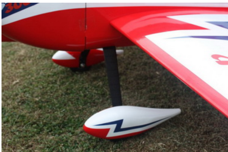
Anodized 6061 Aluminum landing gear
